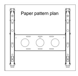
Drill holes on the wall as indicated on the paper pattern plan with a hand drill (power drill) and hammer in the concrete anchors (8) firmly.
